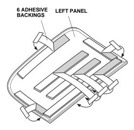
11. Place the left panel on the rear bumper and align it with the masking tape and the mark you made.
