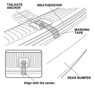
3. Position the center panel on the rear bumper, and align it with the center mark on the masking tape as shown.
