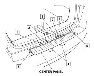
8. Remove the masking tape. Using the rubber roller, apply firm pressure to the center panel, especially at the ends, as shown.
