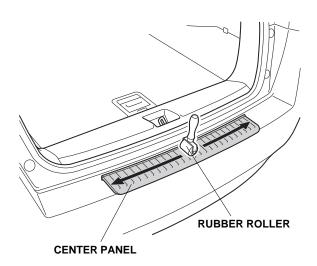
Position the left panel on the rear bumper and align it with the center panel. Attach a piece of masking tape to the rear bumper at the edge of the left panel. Using a marker, mark the masking tape at the measurement shown. Remove the left panel.
