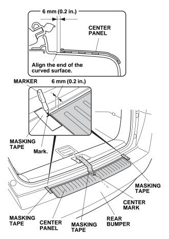
4. Attach a piece of masking tape to the rear bumper at each end of the center panel as shown. Using a marker, measure 6 mm (0.2 in.) and mark the tape as shown. Remove the center panel and the center piece of masking tape.
