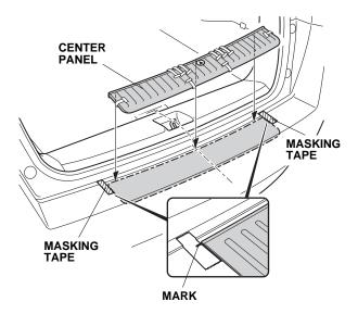
7. While pressing the center panel firmly with the palm of your hand, slowly and carefully remove the adhesive backings in the order shown.
