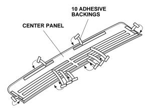
6. Place the center panel on the rear bumper between the two pieces of masking tape at the marks you made.
